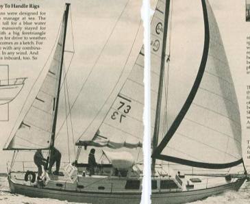
Bill Lapworth gave the 2-46 a 37 1/2-foot waterline and a long shallow keel for exceptional speed and an easy motion at sea.
