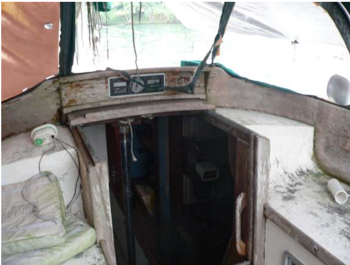
Main companion way with rotten protection. Canvas also need to be renew.
