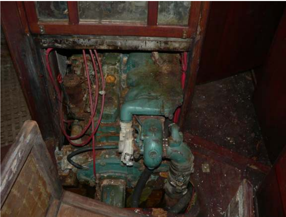
Engine view from aft cabin and some bilge and tanks between galley and salon. We think that the engine is ceased and the best is to changed it, but it maybe serviceable.
