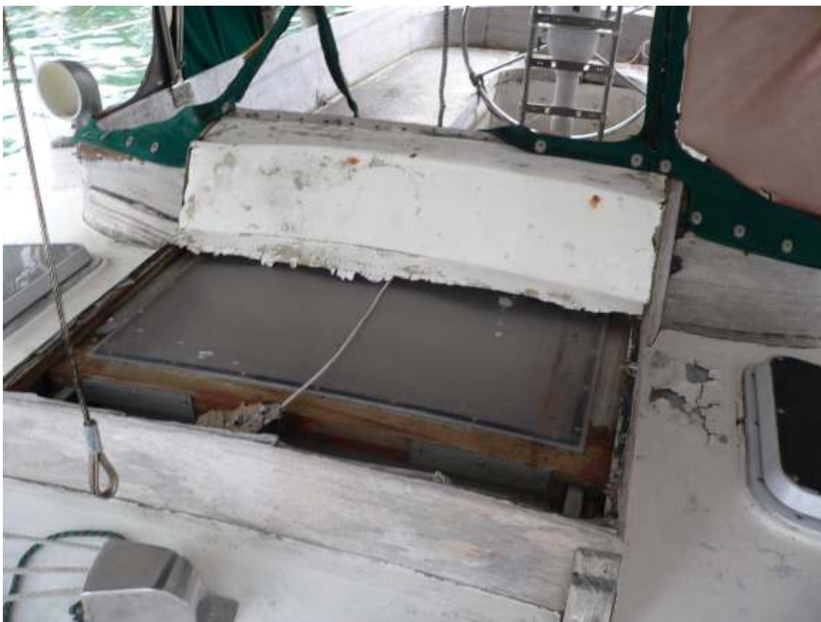
Main companion way with rotten protection. Canvas also need to be renew.
